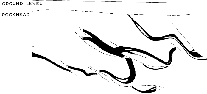
Fig.1 - Section of Big Seam through Llannon Disturbance
